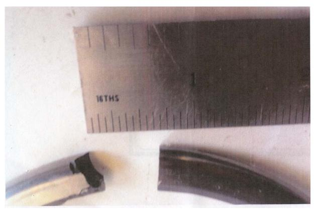
PROPELLERS: McCauley D3A32C406-C, Broken Bearing Race, ATA 6111
